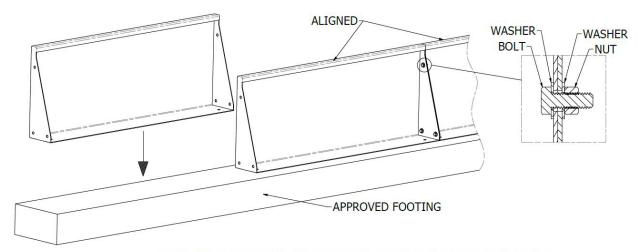
DRY FIT. MARK ANCHOR LOCATIONS BEFORE DRILLING.
